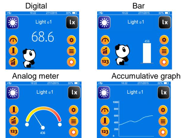
In **experiment record** mode, Panda displays the sampled values of up to two sensors at a time. It records, in its flash memory, the measurements of all its internal sensors (and also external if connected while the measurement is performed). These values can be displayed at any time.
