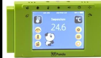
The viewer's screen uses resistive touchscreen technology which reacts to a pressure being applied to the screen – opposed to the more common capacitive screen which requires an electrical conductor to operate. This allows for students to operate the screen even while wearing gloves.
